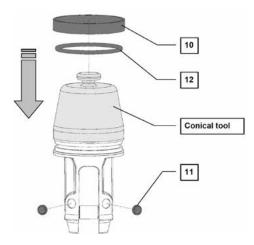
B) Push into its piston seats the P.T.F.E. supports (part N° 11).
