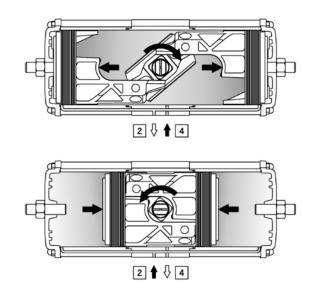
The port 2 is in connection with the cylinder side chambers, supplying the pressurised air in port 2 the standard Double Acting actuator drive shaft rotates counter clockwise to open, while the port 4 is in connection with the intermediate chamber and when pressurised the drive shaft rotates clockwise to close.
