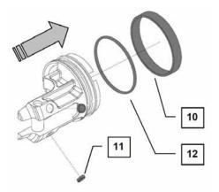
D) When the components are disassembled, they should be properly cleaned, and wear checked prior to being greased and reassembled. In case the sealing parts are too much worn out use new parts from the spare parts kit.
