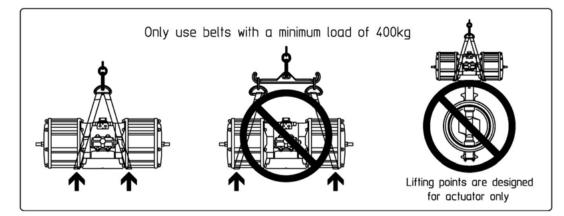
Before performing any installation operation, verify the actuator and valve conditions according to the safety notice above described. Moreover, the utmost clearness is required during valve installation of the air supply connection to the actuator. All the connection parts such as reductions, joints, plates, brackets and equipment must be clean and dirty free.
