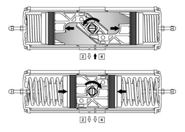
The port 4 is in connection with the intermediate chamber and when pressurised the drive shaft rotate counter clockwise to open.
